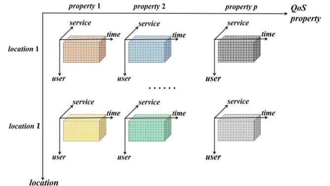
Fig. 2. Structure of a five dimensional QoS data in terms of location, QoS property, user (or client), service, and time period.
