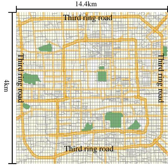
Fig. 4. For each location grid, the transformed BTP dataset surveyed on two things for every time interval: how many people called taxi and how many people got off taxi. We divided the city zone of Beijing within the third ring road into 3600 location grids, each of which is 240m×240m in size. We also divided each day into 144 10-minute time intervals.
